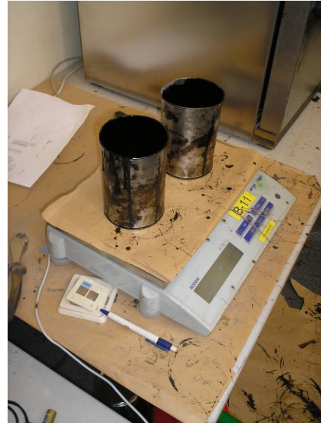
Figuur A4.6: Bitumen invegen
